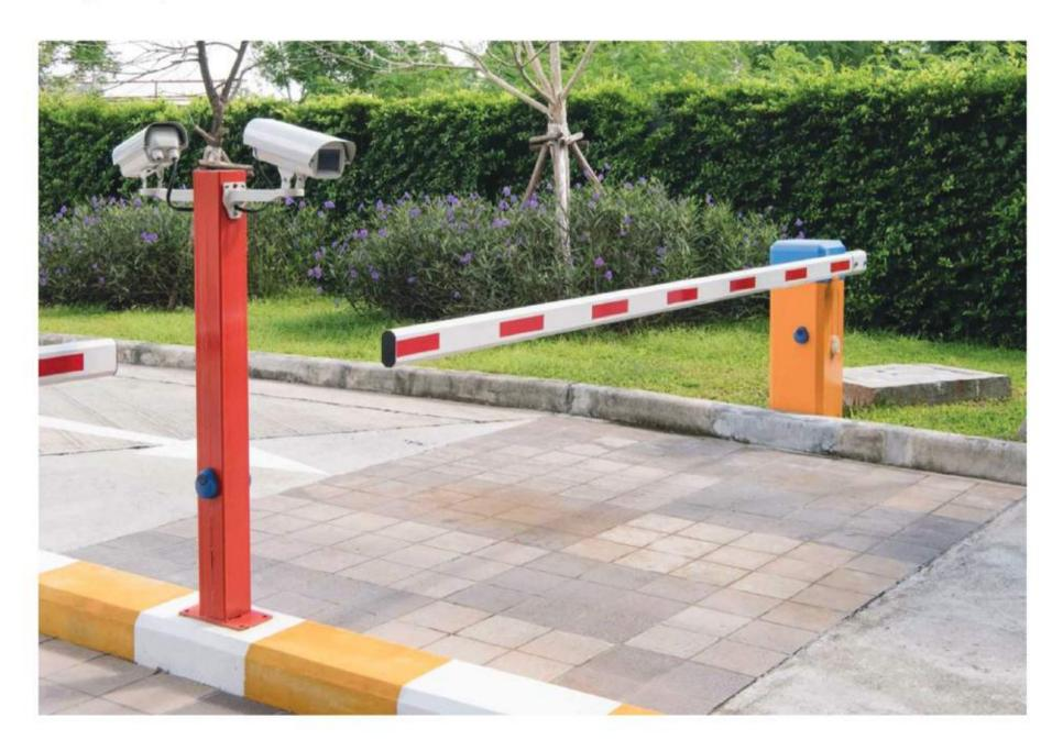
Boom barriers include an inbuilt anti-crush safety device, which suspends the motion of the arm, should it meet any obstruction. Optional beam sensor provides further protection to vehicles. Auto-close of the boom barrier can be programmed through the controller. Duration of fast and slow speeds is programmed at the time of installation, according to the length of the boom and frequency of traffic expected.
